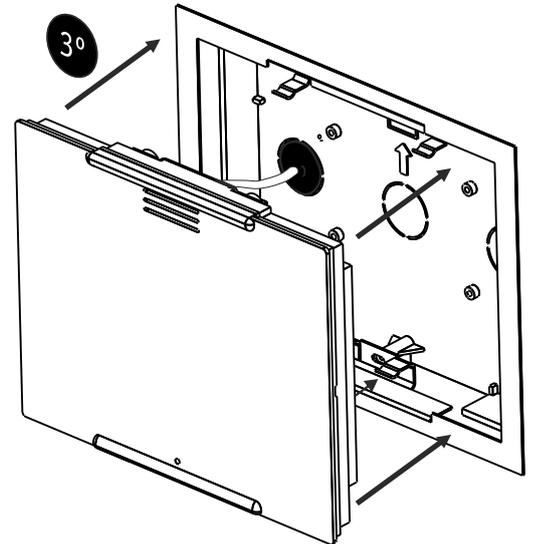
**Note:** When the monitor is placed into the frame, if you feel it is not firmly fixed, bend slightly the fixing points of the frame to increase the fastening.
