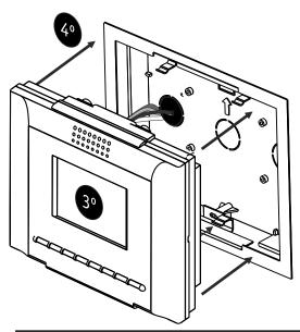
Note: When the monitor is placed into the frame, if you feel it is not firmly fixed, bend slightly the fixing points of the frame to increase the fastening
