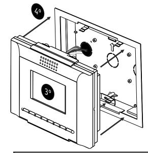
Note: When the monitor is placed into the frame, if you feel it is not firmly fixed, bend slightly the fixing points of the frame to increase the fastening
