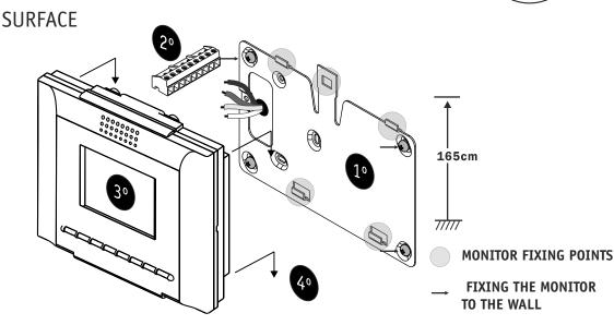
1º- Fix the iron sheet to the wall with the provided screws. The iron sheet allows adjusting little deviations.
