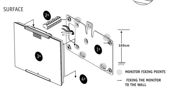
1°- Fix the iron sheet to the wall with the provided screws. The iron sheet allows adjusting little deviations.
