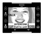
When the monitor receives an intercommunication call, the ring is monotone and in the screen we'll see the number of the monitor which is performing the call.
