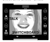
·When the monitor receives a call from a switchboard, everything works as in the panel case, unless that the ring is monotone and the open-door option is not available. If the switchboard has a camera its picture will be displayed on the monitor.
