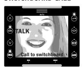
If there is a Switchboard in the installation, it is possible to establish an audio communication with it, pressing **OK** + ( --- ) with the monitor in stand by mode. The conversation length is up to 1m 30s maximum.
