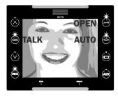
The video can be activated with any panel or 'smart' camera in the installation by pressing ( ). It can be done even in the conversation stage.
