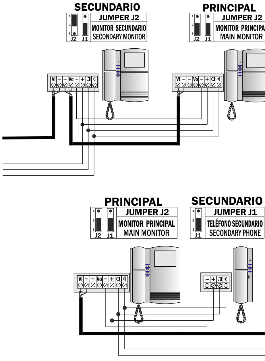
**SIN COAXIAL***Monitor Compact Digital***INSTALACIÓN DE MONITORES EN CASCADA**
