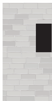
Colocar caja de empotrar Place mounting box
