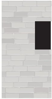
Colocar caja de empotrar Place mounting box
